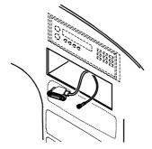
Insert the DIN/ISO console into the ISO slot, and secure by bending the locking tabs. Note that the spare slots are in the base of the frame. Ensure that the frame is firmly placed.
